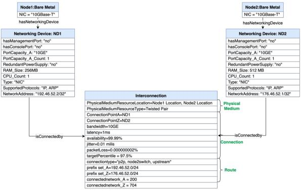
Figure 6: Example of interconnection for two nodes.
